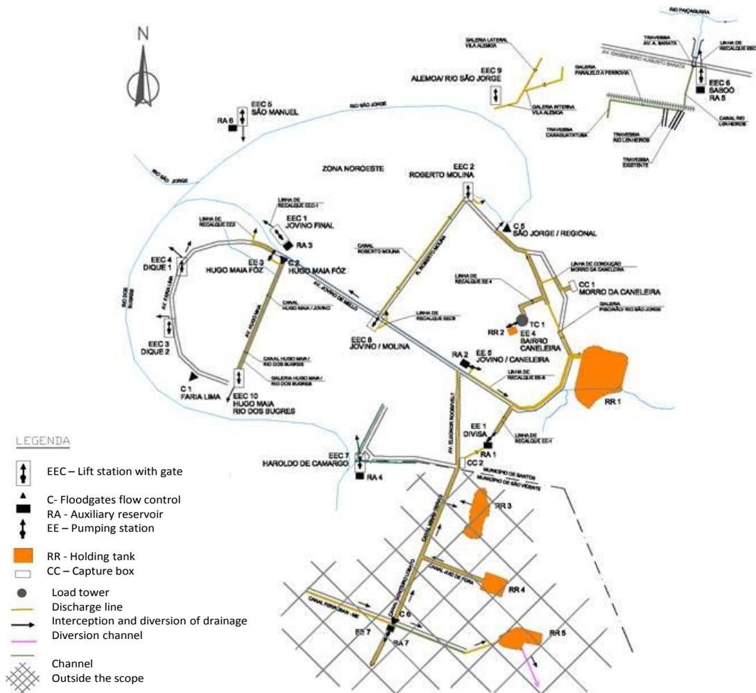
**Figure 2.12 Macro-drainage system for the Northwest Zone of Santos proposed under the Santos Novos Tempos Program. Source: MC Consulting, 2012.**
