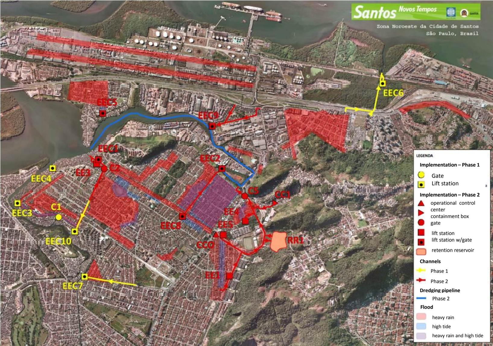
Figure 2.10 The new drainage system in the Northwest Zone of Santos, Source: provided by MC Consulting.
